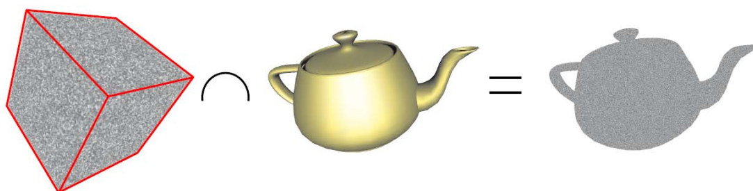
Figure 4: The polygonal model is carved out of a 3D solid noise texture
